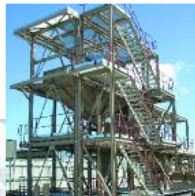
One of the two secondary Dense Medium Cyclone circuits for the Vele wash plant in construction at supplier factory.
